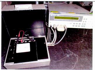
Fig.4: Insulation resistance test
