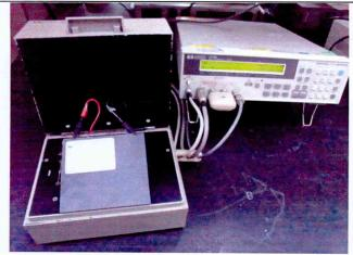
Fig.3: Insulation resistance test
